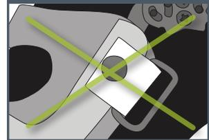
**\*Please note that the "D-Rings" for the two center straps face forward to prevent pinching. DO NOT rotate these to face rearward.**
